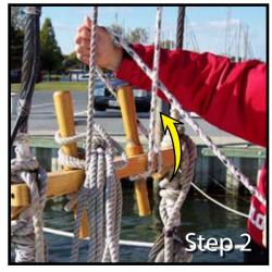
Step 2: Take the sheet up on the right side and around the back of the upper end of the pin.
