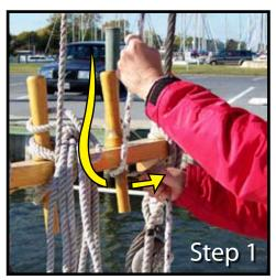
Step 1: Bring the jib sheet down on the left side and around the back of the lower end of the pin.
