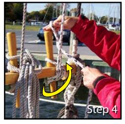
Step 4: Give the line a counterclockwise half twist and form a loop. Place it over the top of the pin so that the beginning of the loop comes diagonally up and across the front of the cleat and lies over the end of the line, which should lie parallel to the diagonal wrap below it.
