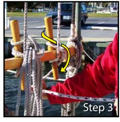
Step 3: Cross the line over the front of the pinrail and bring it down on the right side, taking it behind the lower end of the pin from right to left.
