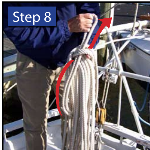
Step 8: Take the doubled end under the FIRST pass you made over the coil in Step 3.
