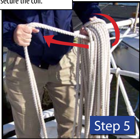
Step 5: Bring the doubled end through from the back to the front of the coil.
