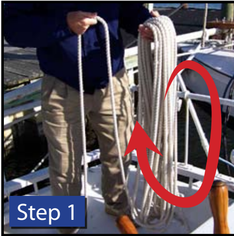
Step 1: Coil the main sheet clockwise, holding it in your left hand and coiling with your right, in very large loops to handle the length of the line.
