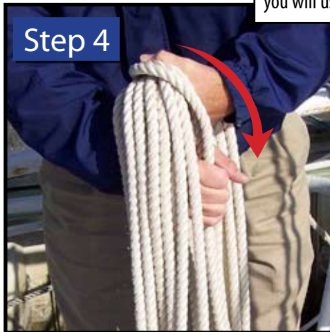
Step 4: Reach your right hand through the coil and take hold of the doubled end.
